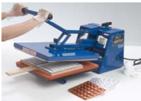
Figure 2 Manual Heat Sealer
